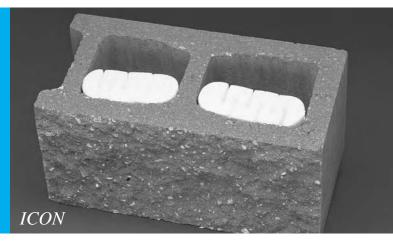
**Composition and Materials: ICON** Inserts are individually molded from expandable polystyrene in a minimum density of 1.3 lbs. per cu. ft. Inserts are packaged at the point of manufacture in heat-sealed, clear polyethylene bags.
