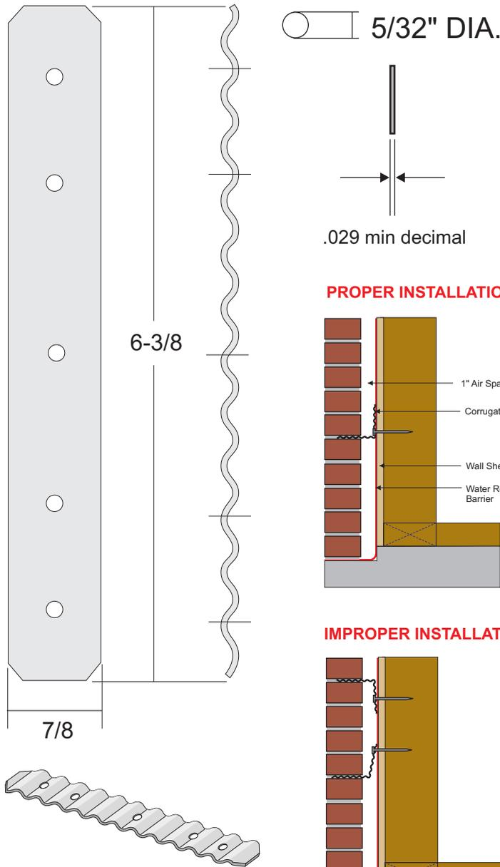
**MATERIAL:** 22 ga. (.029 min decimal) HDG Galvanized - ASTM A 153 Class B-2. Also available in hot dip galvanized after fabrication (in accordance with ASTM A153 B3) and stainless steel (type 3042B) for optimal corrosion resistance. Stainless steel is absolutely best material for longevity.
