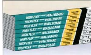
Designed for use in radius walls and ceiling construction. I can be used for both concave and convex surfaces. 1/4" High Flex is typically applied in double layers. Consist of a fire resistive gypsum core encased in heavy, natural-finish paper, and long, slightly tapered edges.
