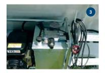
STEP 3: Using the electric start or manual pull start, turn on the gas engine. Then engage the augers by using either the switch on the extension cord or the switch mounted on the power pack. Verify the unit is operating properly. If equipped with the electric power pack, make sure the main power switch is on in lieu of starting the gas motor.
