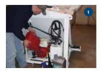
STEP 1: Check all fluids in the power pack. Motor oil should be 10W-30. Hydraulic oil tank should contain 5 to 6 gallons of standard hydraulic oil and gas tank should be filled with unleaded gasoline. Make sure the battery and hydraulic hoses are connected.
